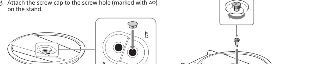
You can also use a coin to tighten the screw.
